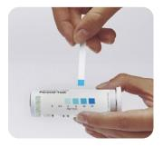
After the specified reaction time (maximum one minute), compare the color of the reaction zone with the color scale printed on the tube label to determine the concentration.
