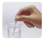
Dip strip into the test solution to wet reaction zones and remove excess liquid.
