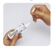
Remove one MQuant® test strip from the protective tube.
